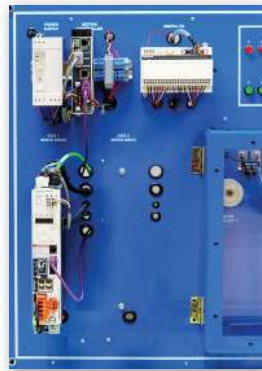
890-MCSE1's Motion Controller, Digital I/O, and Servo Drive
