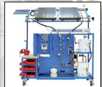
Open-Loop Drainback System
