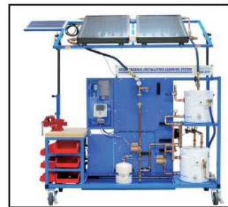
Closed-Loop Drainback System
