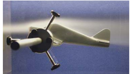
SMOKE TRAIL AROUND THE LOW WING AIRCRAFT MODEL
