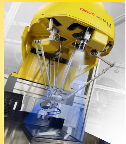
i RVision provides error proofing guidance and part location
