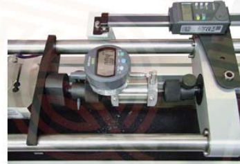
Optional Extensometer (SM1002a) fitted to TL specimen
