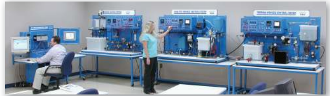
T5552, T5553, and T5554 connected and controlled by the 890-PEC-B (left)
