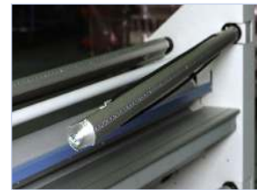
Cantilevered Supply Shaft*
